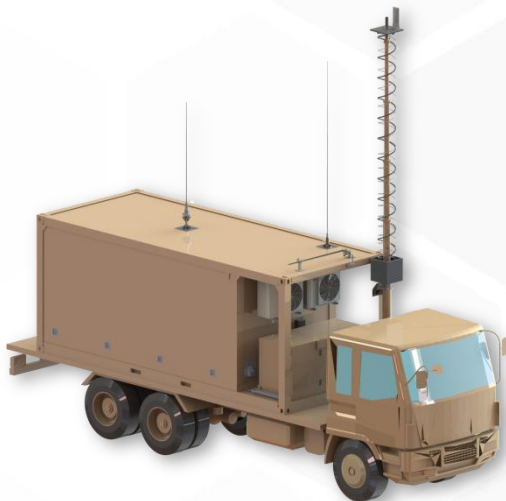
Field deployed Tactical Operations Control Centre
